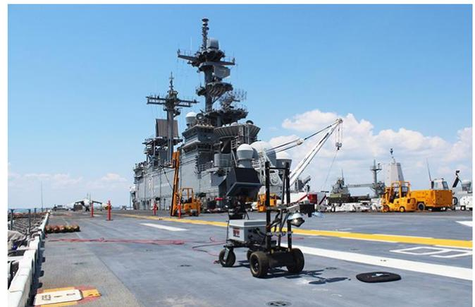
**The Infrared Coating Inspection System (IR-CIS) inspects the flight deck of an amphibious assault ship to detect defects that may result in damaging conditions for aircraft. (Fuchs Consulting, Inc. photo)**
